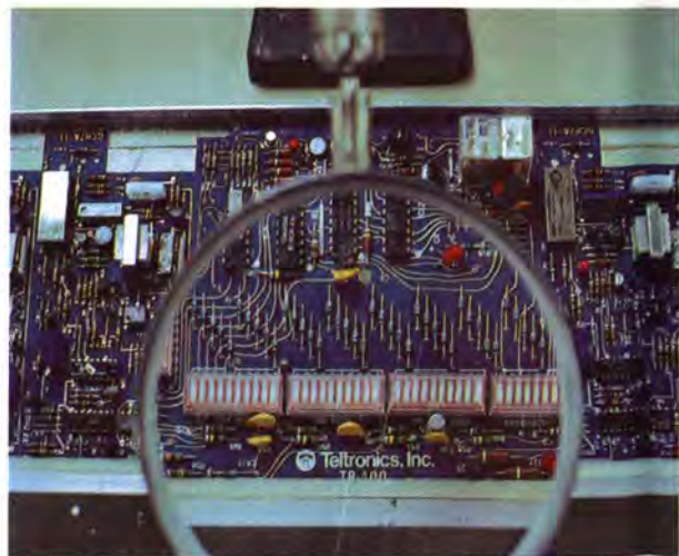
The TR-400 toll restrictor, a Brand-Rex telephony product, limits choice of dialings to prevent unauthorized calling. (Photo: Richard Alcorn, New York)
