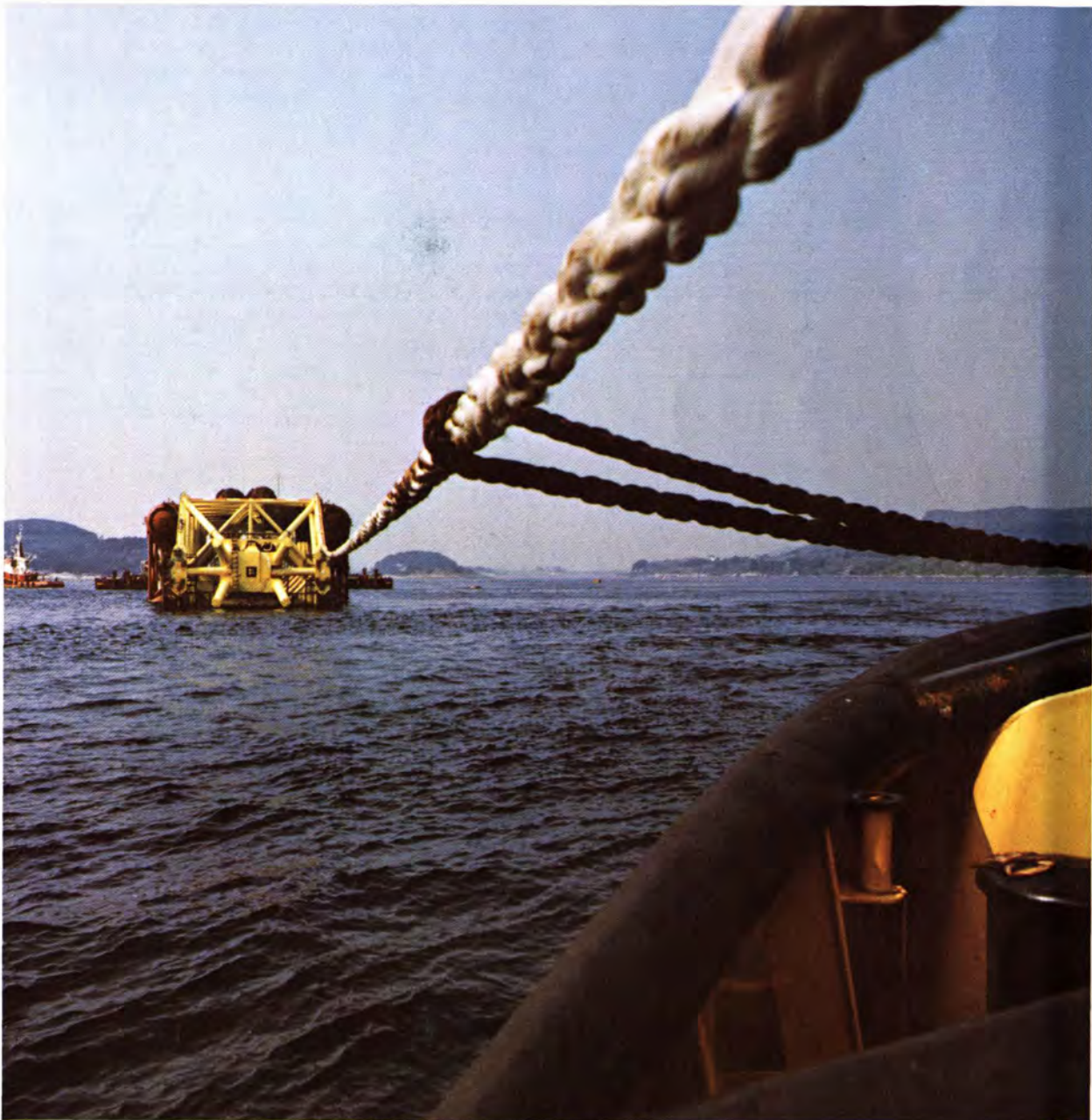
An element of the tow connection, this so-called spring composed of polyamide (nylon) yarns serves to absorb shock loads. (Photo: Pim Korver, Rotterdam)
