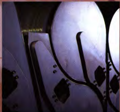
Spinning of the Twaron® yarn, followed by drying of the product on big drums.
