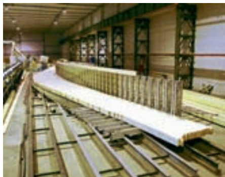
Fig.1 Manufacturing of arched long-span laminated beams.
