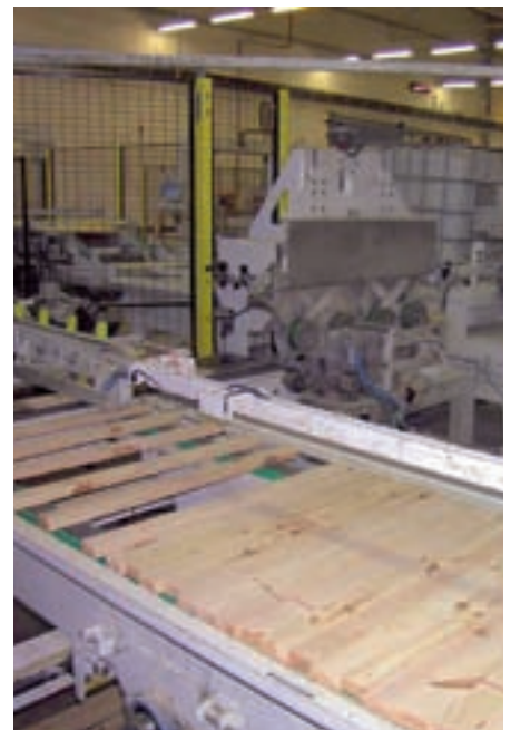
Panels with adhesive applied are fed continuously into the press.
