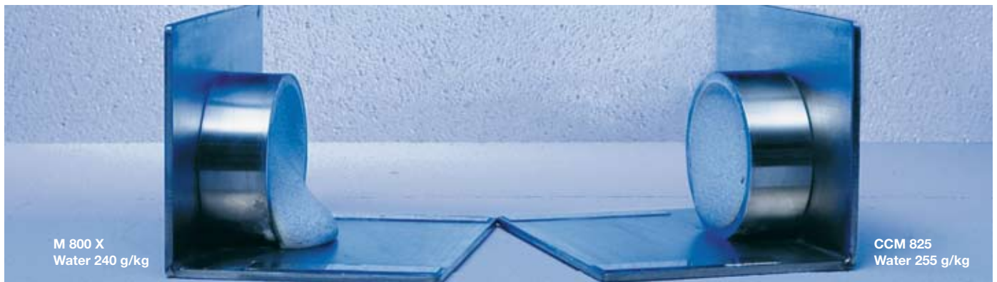
Difference in consistency in a standard CTA formulation between a CCM grade and a standard grade.
