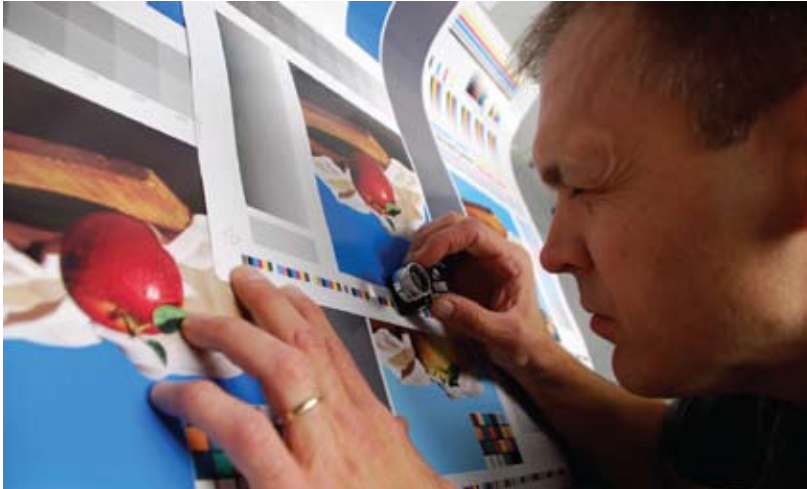
Dale Kohl, Appleton Coated, technical services representative, inspecting the color bars of a test print to insure proper ink and water balance of the Komori press
