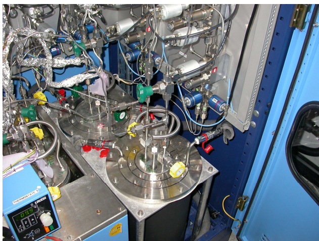
Figure 5. Two 8 l cylinder plus Heat Exchangers in use with an Aixtron 200 machine.
