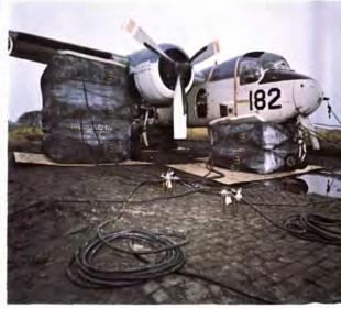
Inflatable cushions of rubber-coated rayon fabric jack up plane for field repairs to landing gear.
