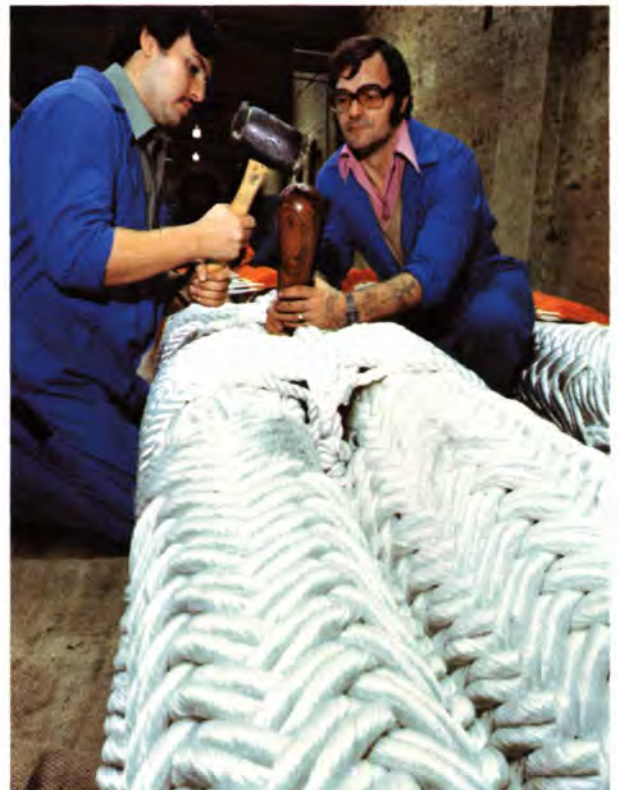
Enka's nylon 6.6 yarn was used in making double ropes, measuring 110 m long and twice 24 cm across, with an assembled breaking strain of 2,400 metric tons. This largest and strongest nylon rope type in the world is to serve in temporary mooring systems for oil rigs.
