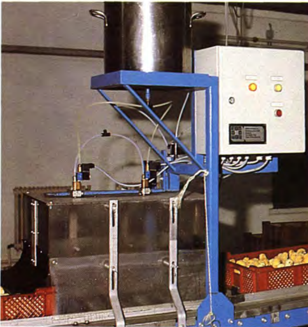
Automatic spray vaccination of day-old chicks with Nobivac® IB vaccine to procure immunity from infectious bronchitis.
