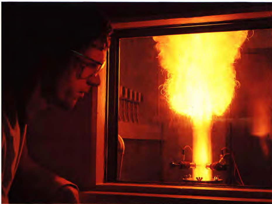
In the chemical division's new safety laboratory at Deventer, the Netherlands, tests are constantly conducted to determine safe handling procedures for organic peroxides.
