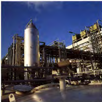
Receiver vessel used in separating chlorinated hydrocarbons from plant effluent at Diosynth, Oss, the Netherlands.
