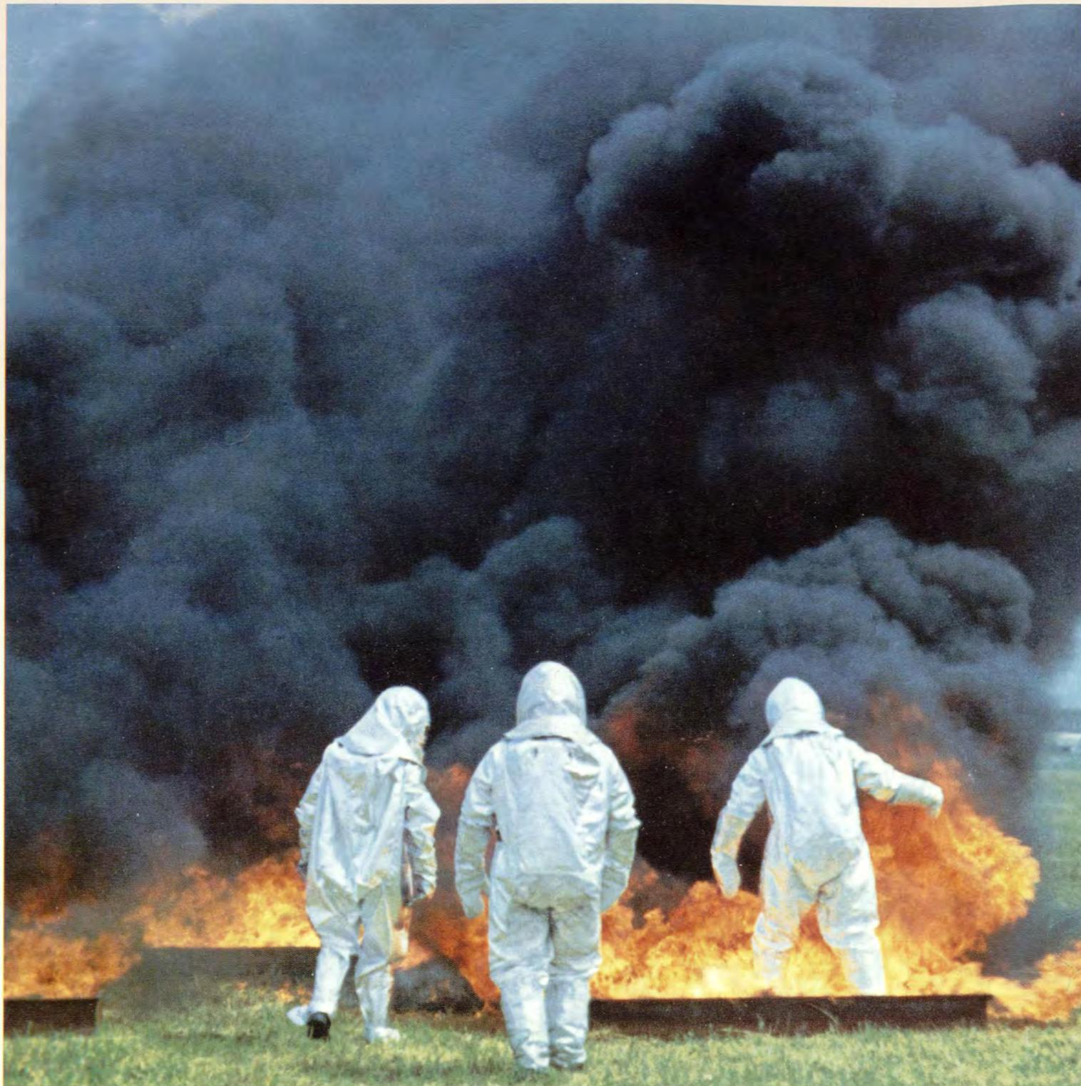
ENKATHERM<sup>®</sup>, developed by Enka Glanzstoff, is a new, non-flammable and non-melting fiber material with a flame resistance exceeding 1,000 °C. It is eminently suitable for heat-resistant and fireproof garments.
