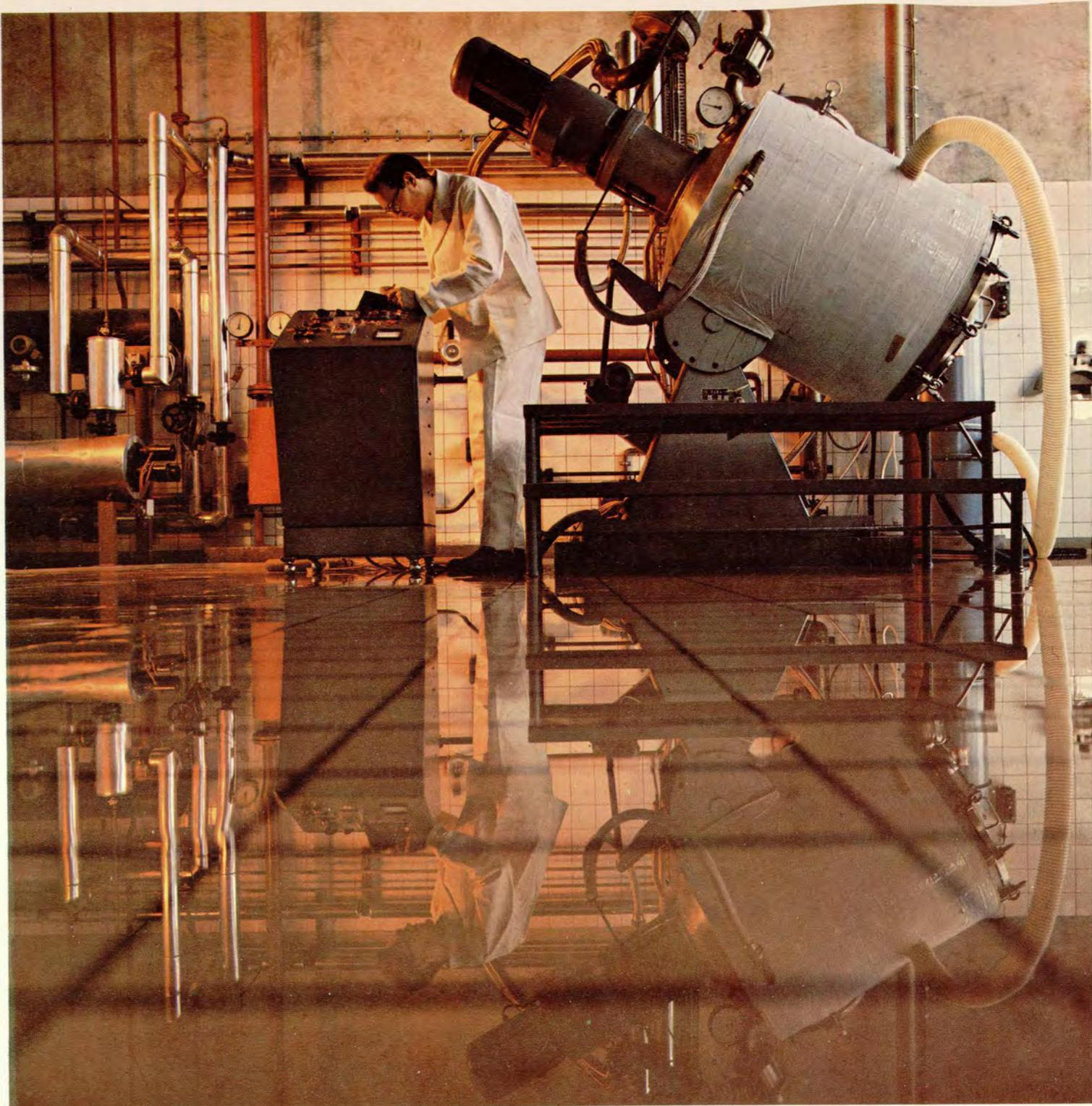
n.v. Organon has acquired a topo granulator for pretreatment of pharmaceutical substances to be included in tablets. This newly developed apparatus greatly simplifies the production process.
