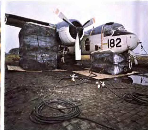
*Inflatable cushions of rubber-coated rayon fabric jack up plane for field repairs to landing gear.*
