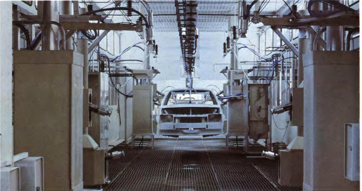
Application on the assembly line of our primer-surfacer which contains no organic solvents.
