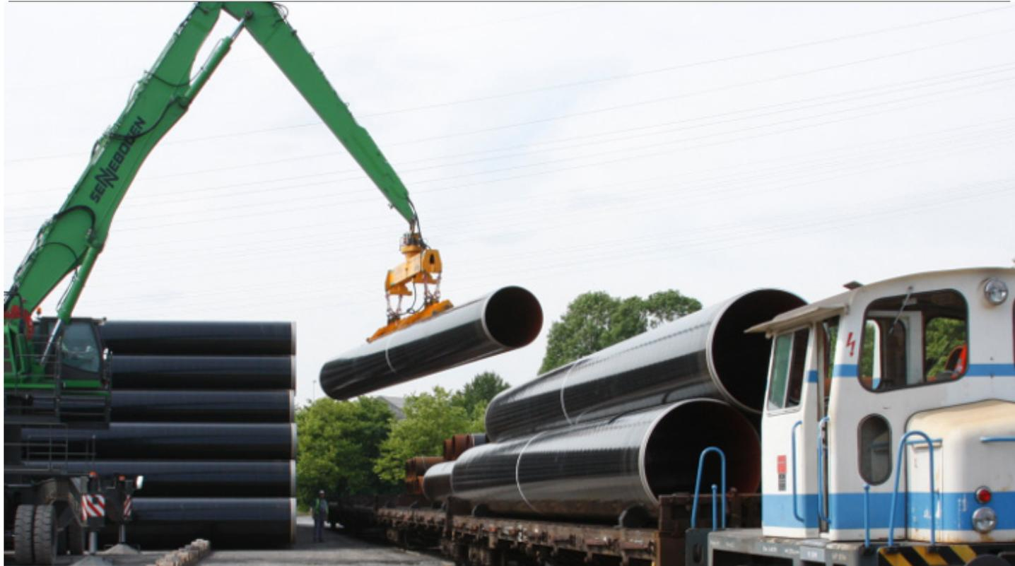
AkzoNobel provided powder coatings for the 1,223-kilometer long Nord Stream gas pipeline. Due to be operational in 2012, the pipes have been coated with a Resicoat primer for a three-layer system. In total, 1,500 tons of coatings were delivered for the project.
