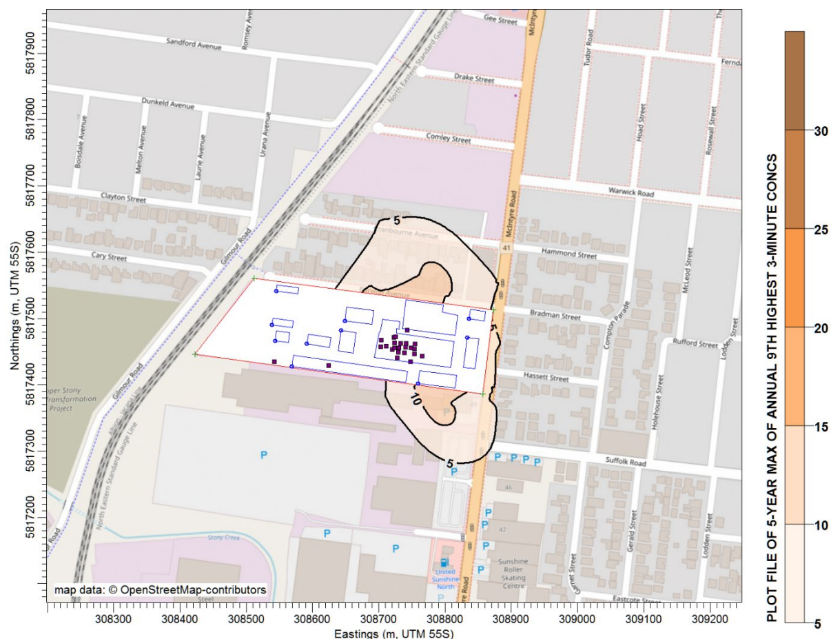
Figure 8: Scenario 2 maximum 3-minute ground level odour concentrations.
