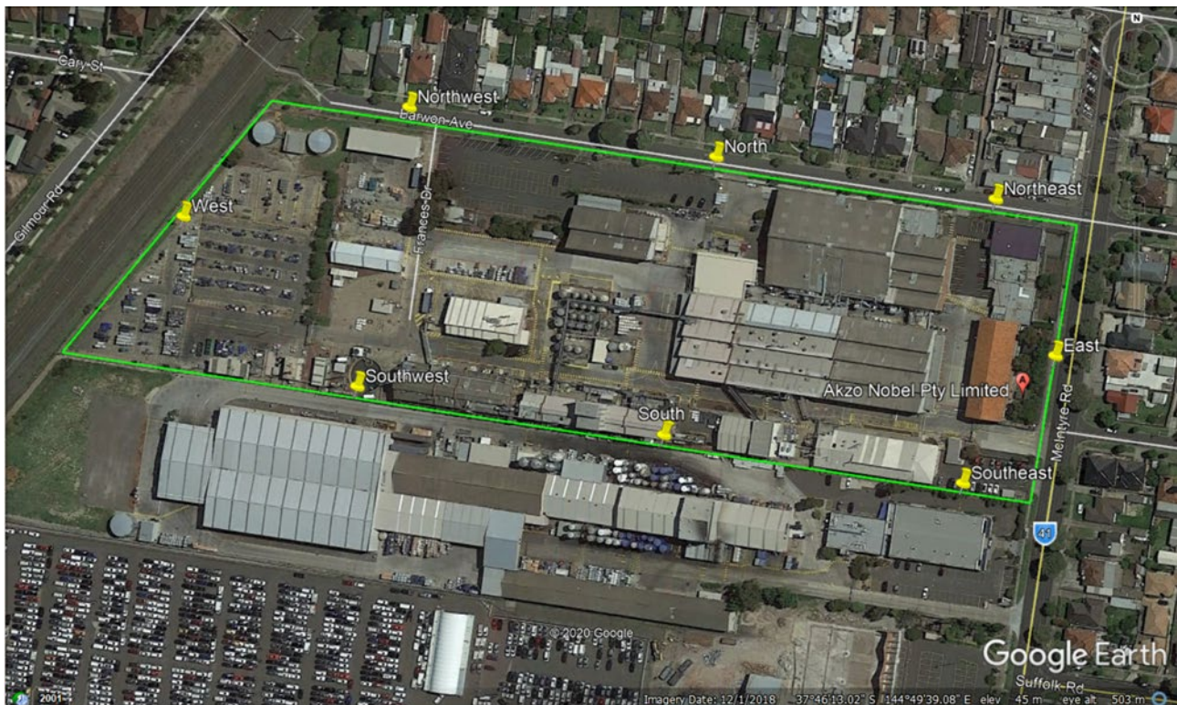
Figure 2: AkzoNobel property boundary (green) and VOC monitoring locations (labelled pins).
