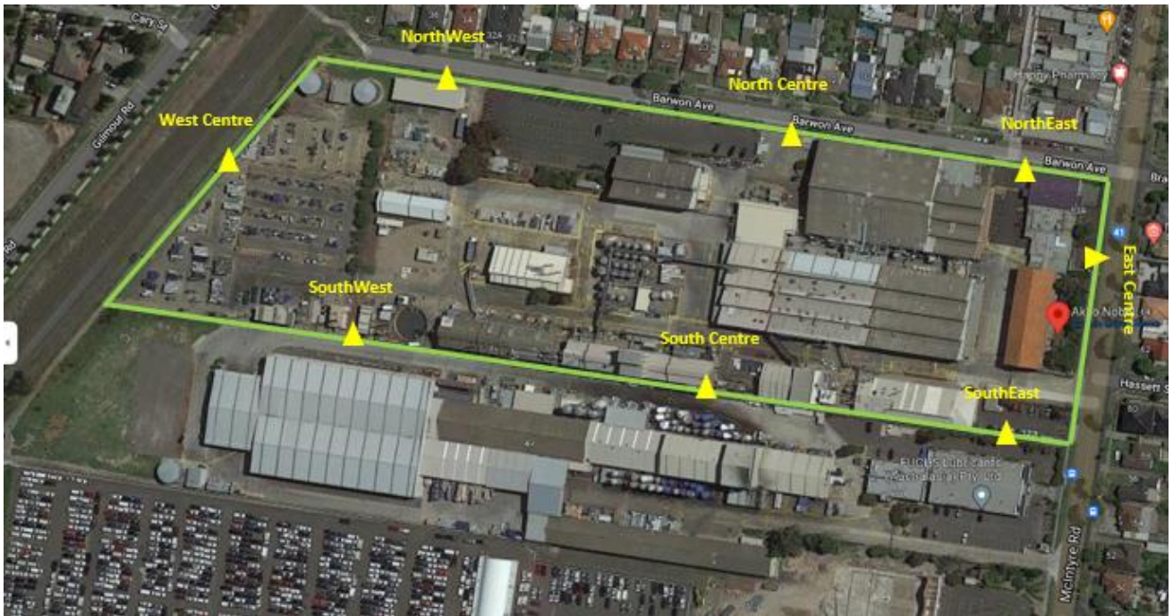
Figure 1: Boundary odour monitoring route
